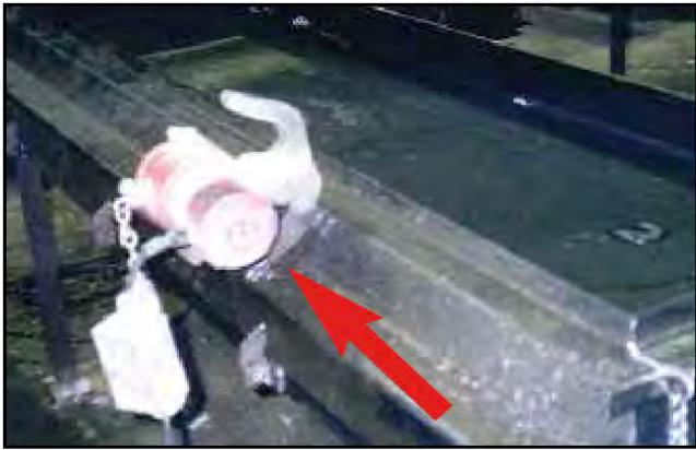
Model US-450 on wedge-bracket for vibrating lid on burial vault form.
