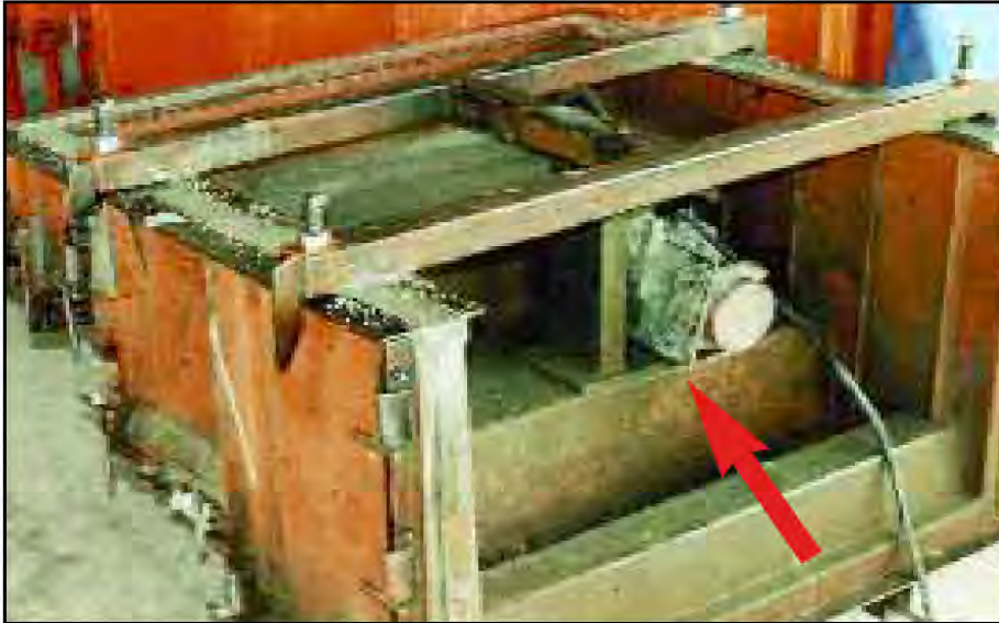
3-Step Form using US-900 Electric with UW-2 Wedge Bracket.
