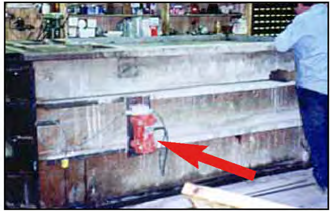
Model US-1600 permanently mounted on 5500 lb. mold.
