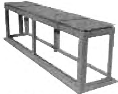
12' long vibrating table to handle multiple forms
