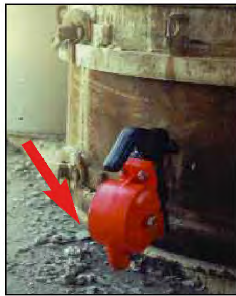
Silent pneumatic turbine model VS-510 on wedge bracket on well liner form.
