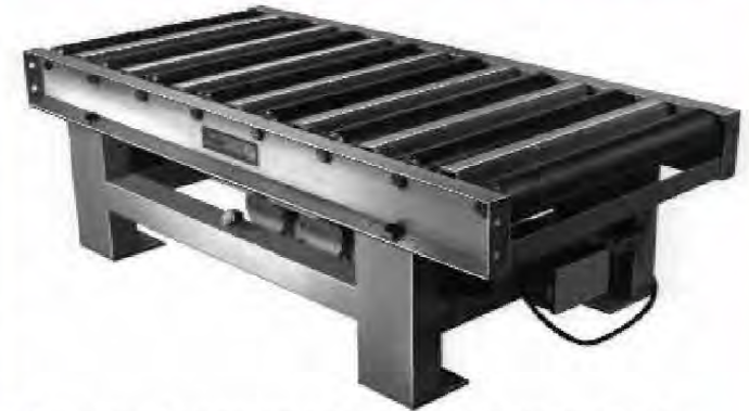
Vibrating roller conveyor for increased production in cultured marble factory.
