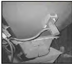
Weigh Batcher with Model 55-1-1/2 Piston
