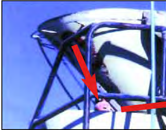
VIBCO VS-250 air vibrator mounted on the charge hopper of a front discharge mixer truck. (Complete kit available.)
