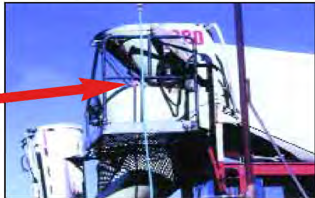
VIBCO VS-250 air vibrator mounted on the charge hopper of a front discharge mixer truck. (Complete kit available.)
