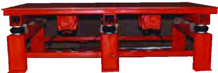
vibrating table with electric vibrators to handle a long 10,000 lbs. concrete form.
